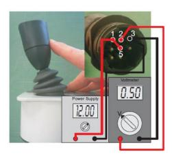
Power supply positive on pin 1 and 5 on the connector
