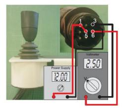
Power supply positive on pin 1 and 5 on the connector
